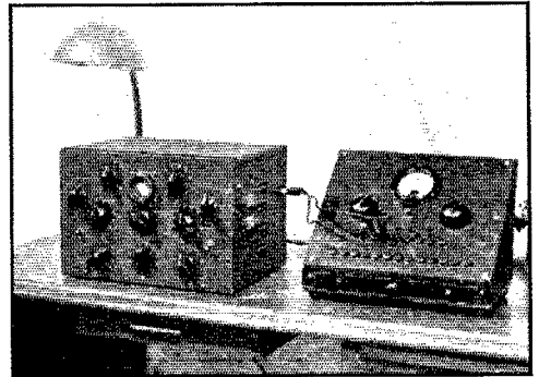
Fig. 2 — The set-up used in making the measurements. The oscilloscope on the left is connected to the d.c. voltmeter at the right by two flexible leads. Reading from left to right on the voltmeter, the controls are: range switch, r.m.s. toggle switch, and the potentiometer which controls the d.c. output.
